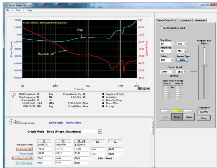
Figure 9. Bode plot of main and receiver port isolation showing test parameters, cursors and annotations.
