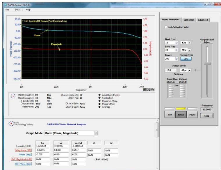
**Figure 7. Graphical output (bode plot) for EUT terminal and receiver port insertion loss.**
