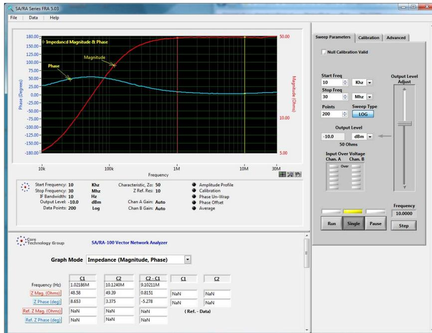
**Figure 3. Graphical output for the EUT terminal impedance showing magnitude and phase.**
