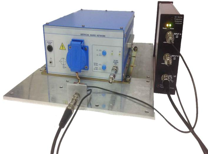
Conducted emissions is a measure of the amount of Electromagnetic Interference (EMI) that is conducted from a unit under test (EUT) to the outside world via the power cables. A Line Impedance Stabilization Network (LISN) is used for conducted emissions testing, and is inserted between the power mains and the EUT.
