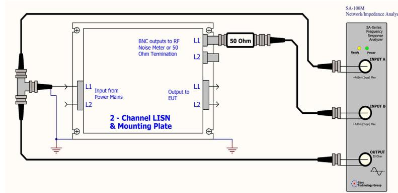
Figure 8. Test setup using the SA-100 measuring main and receiver port isolation.
