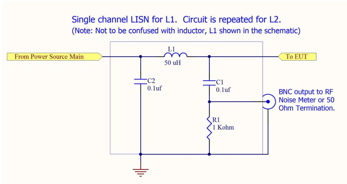
**Figure 1. Circuit model of an LISN as outlined in ANSI C63.4-2003.**
