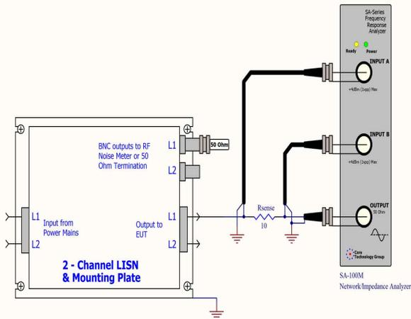
**Figure 2. Test setup for measuring the EUT terminal impedance.**
