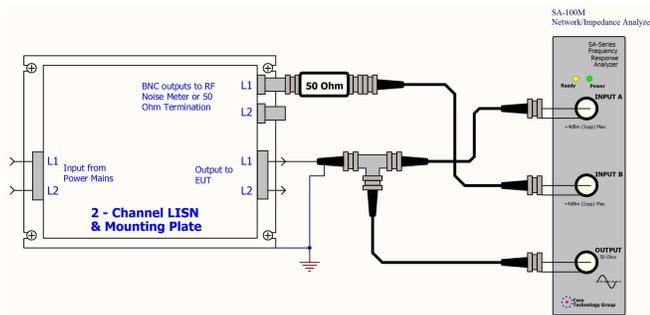
**Figure 6. Test setup for EUT terminal and receiver port insertion loss (transfer function).**
