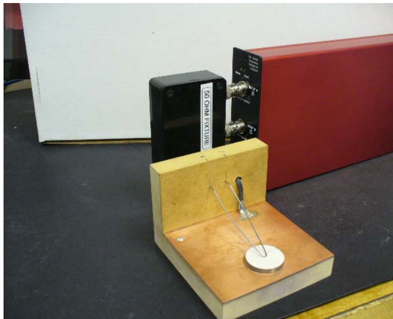
Figure 5. Test setup shown with fixture connected to the SA Series Vector Network Analyzer with a disc type element ready for testing.
